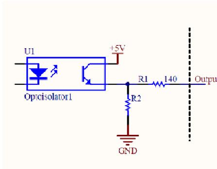
Figure 8 PLC digital output equivalent circuit
