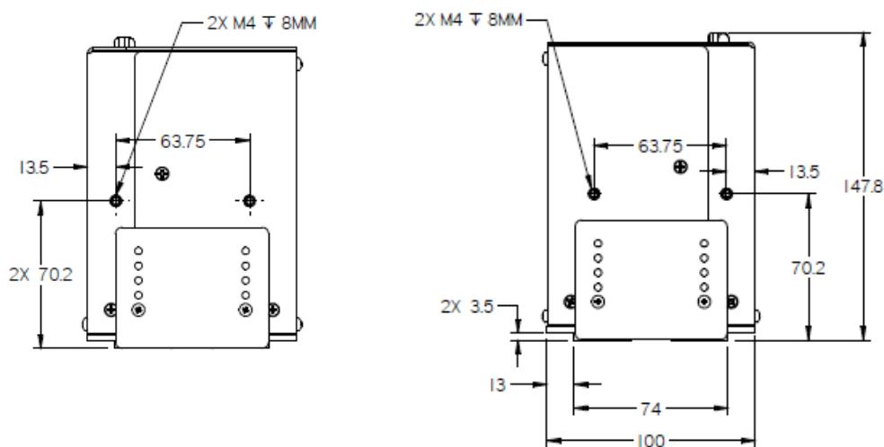
Figure 4 UV LED Head Side Dimensions (both models)
