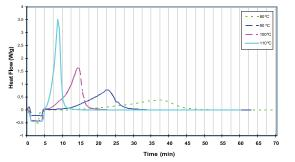
Different exotherm peaks for a typical epoxy at 80°C, 90°C, 100°C and 110°C.
