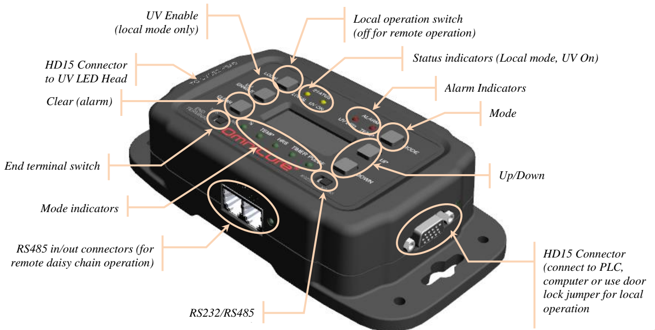
Figure 4 PLC2000 Remote Control Console
