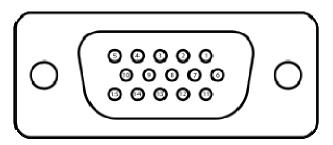
Figure 6 PLC Connector (looking at UV Head)
