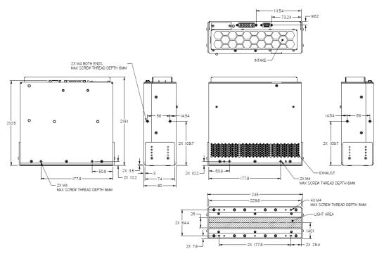
Figure 4 AC8225 UV LED Head Mechanical Drawings
