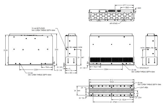
Figure 3 AC8300 UV LED Head Mechanical Drawings
