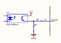
Figure 7 PLC Digital Output Equivalent Circuit
