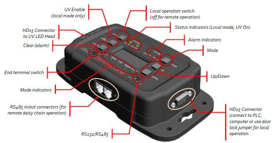
Figure 2 PLC Console (PLC2000 Remote Control Console shown)
