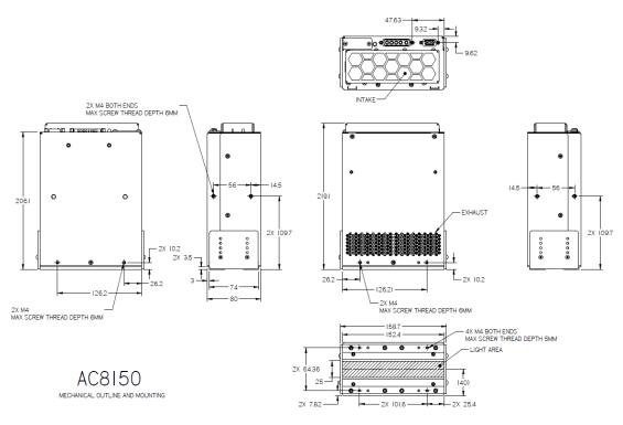
Figure 5 AC8150 UV LED Head Mechanical Drawings
