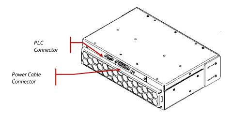
Figure 1 UV LED Head Connection Ports
