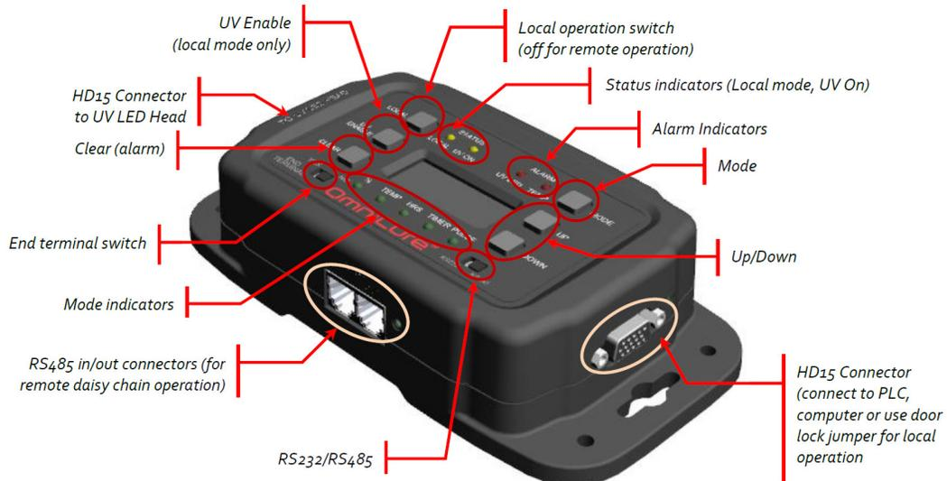
Figure 2 PLC Console (PLC2000 Remote Control Console shown)
